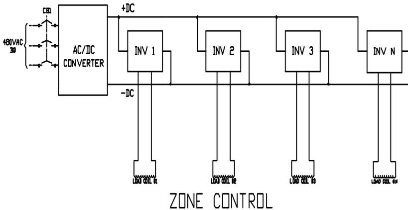
Typical Zone Control Configuration, DC Section – 2000 kilowatts, Inverter 1, up to 1500 kW, Inverter 2, up to 750 kW, Inverter 3, up to 750 kW, Inverter 4, up to 750 kW
