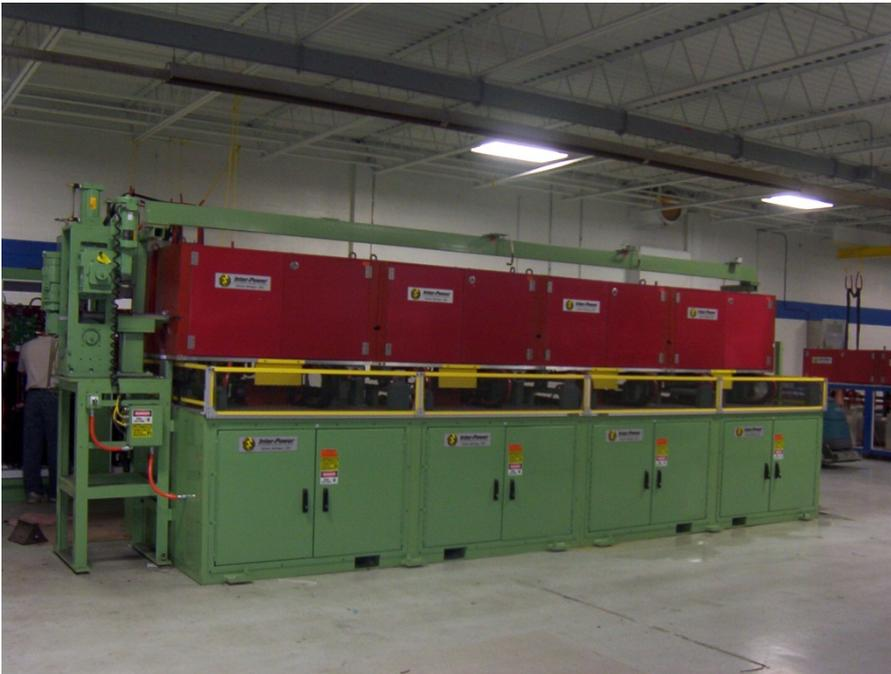
Four Zone Induction Heater with Coil Shuttle. Each Coil is Independently Controlled and there are Two Mounted Sets of Induction Coils for Coil Changeover by Selector Switch.
