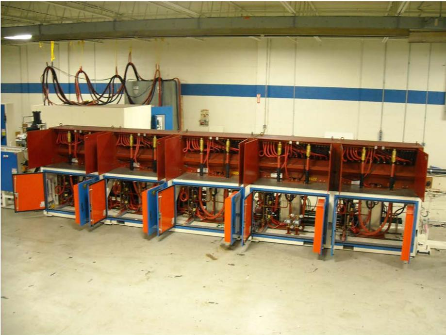
Five Zone Induction System with Doors Open to Inverter Sections.
